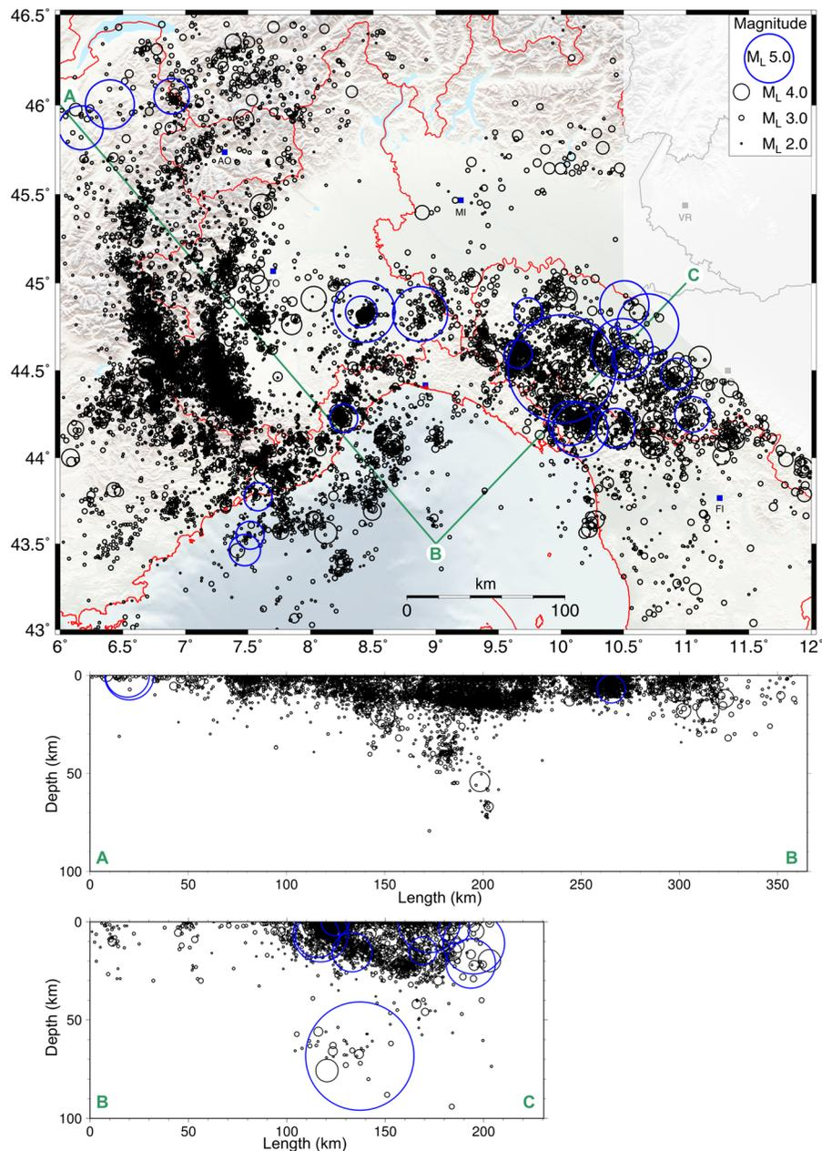
**Fig. 4** Map and cross sections showing the distribution of earthquakes with  $M_L \geq 2.0$  recorded in the last 30 years from the RSNI network. Only earthquakes with horizontal and vertical location
