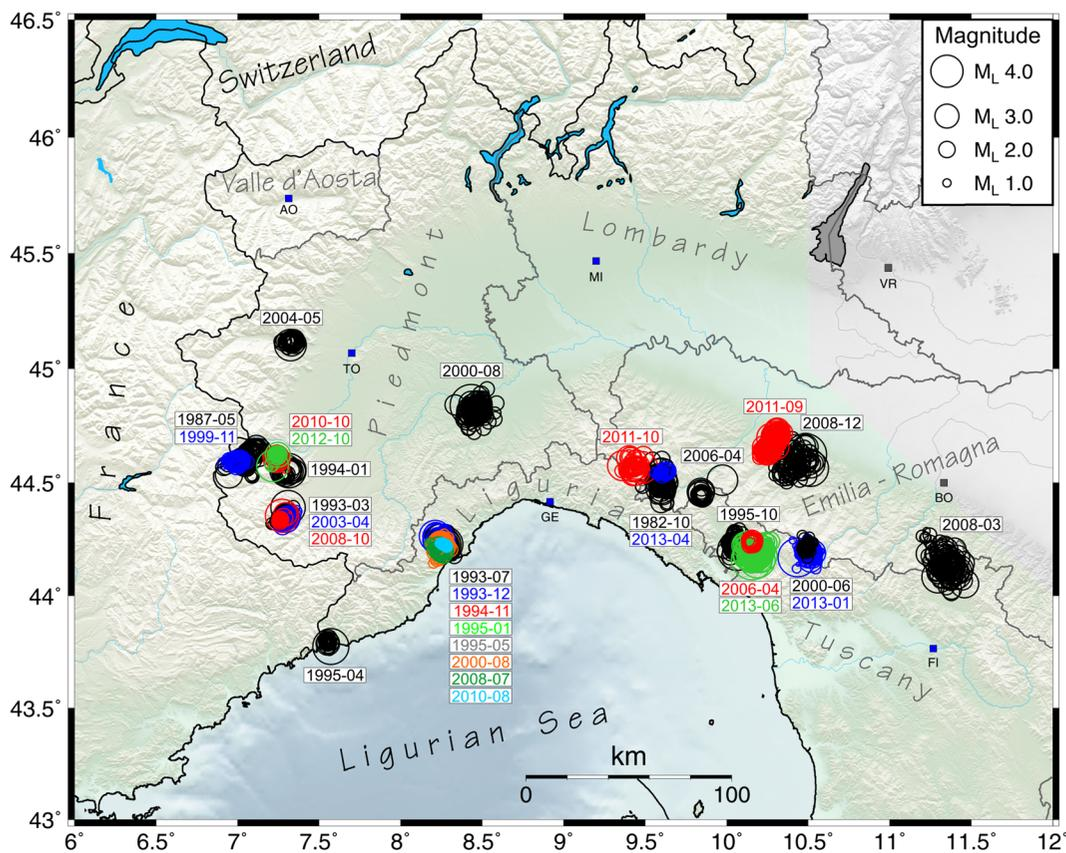
**Fig. 8** Map showing the locations and the times of occurrence of the most significant (more than 20 events in 24 hours) seismic sequences that occurred in Northwestern Italy in the last 30 years
