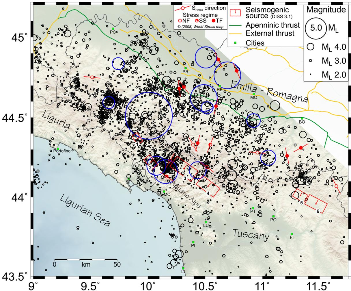
**Fig. 6** Seismicity in the Northern Apennines superimposed on the main seismogenic sources (DISS 3.1, DISS Working Group 2010) and geological features (modified from Bigi et al. 1990) of the area. Stress regime and directions of the maximum horizontal
