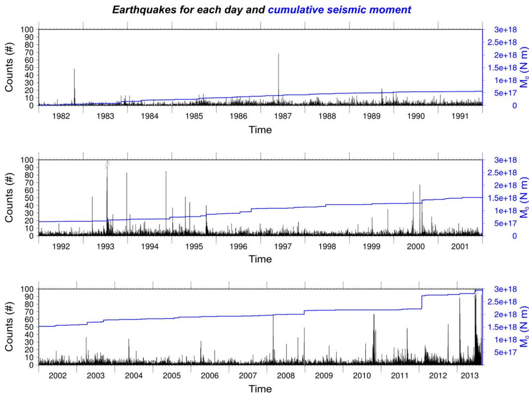
**Fig. 7** Histograms showing the number of events per day as recorded by the RSNI network in the last 30 years with diagrams of the cumulative seismic moment ( $M_0$ )
