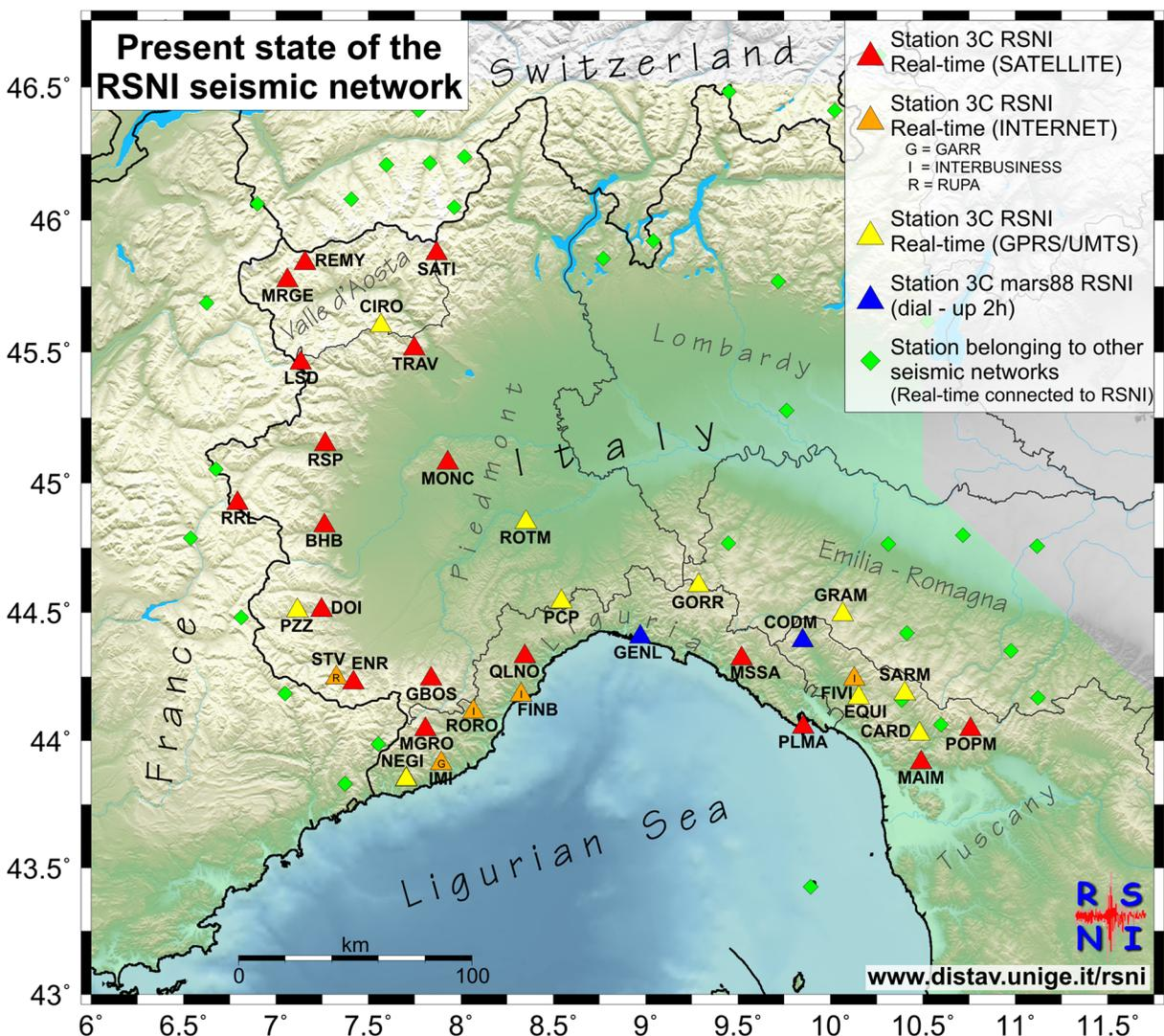
**Fig. 2** The actual geometry of the RSNI seismic stations installed in Northwestern Italy belonging to the RSNI seismic network and other interconnected surrounding networks. The seismic stations are differentiated depending on the type of transmission system
